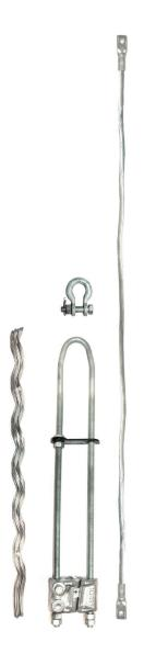
The FIBERLIGN Dead-end is designed to terminate Optical Ground Wire (OPGW) while minimizing any compression stresses that may be transferred to the core or optical elements within. The combination of retaining rods, wedge and housing distribute axial and compressive loading over a large area of the OPGW cable. Left-hand or right-hand lay style is provided to suit left-hand or right-hand lay OPGW respectively.
