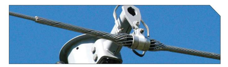
The FIBERLIGN Suspension provides superior cable and fibre protection at the support point. The combination of structural reinforcing rods, outer rods, 'boltless' housing and resilient inserts reduces compression, clamping, and bending stresses on cable. Negative effects of wind-induced cable motion, such as aeolian vibration, galloping, and wind sway are also minimized.
